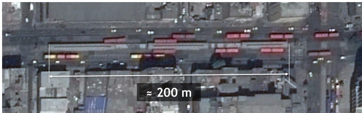
Figure 23: A large station with three sub-stops in Bogotá's TransMilenio system occupies a length of approximately 200 m.
