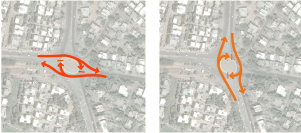
Figure 16: Signal phases for a squareabout intersection.
