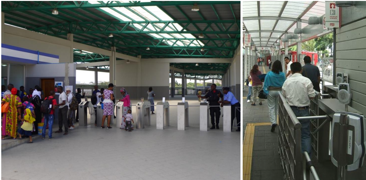
Figure 39: Off-board fare collection is used across many high capacity BRT systems, including systems in Dar es Salaam (left) and Mexico City (right).
