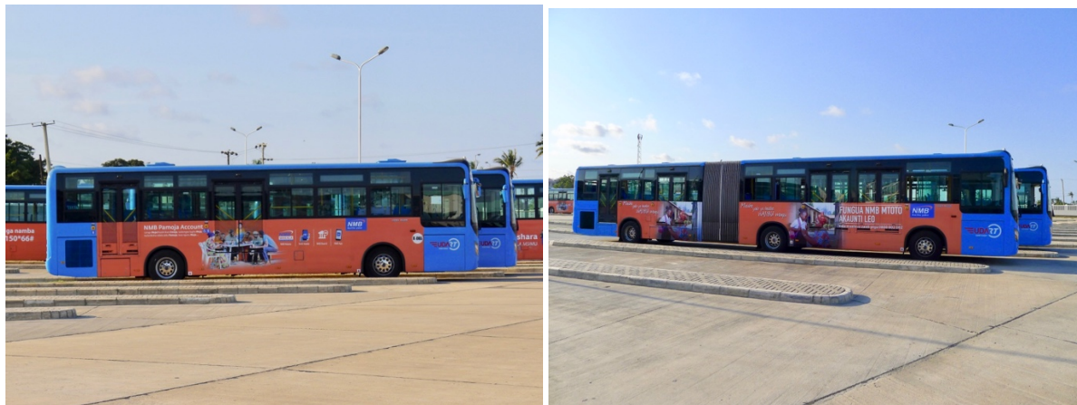
Figure 35: A 12 m standard BRT bus (left) and an 18-m articulated bus (right) in Dar es Salaam.
