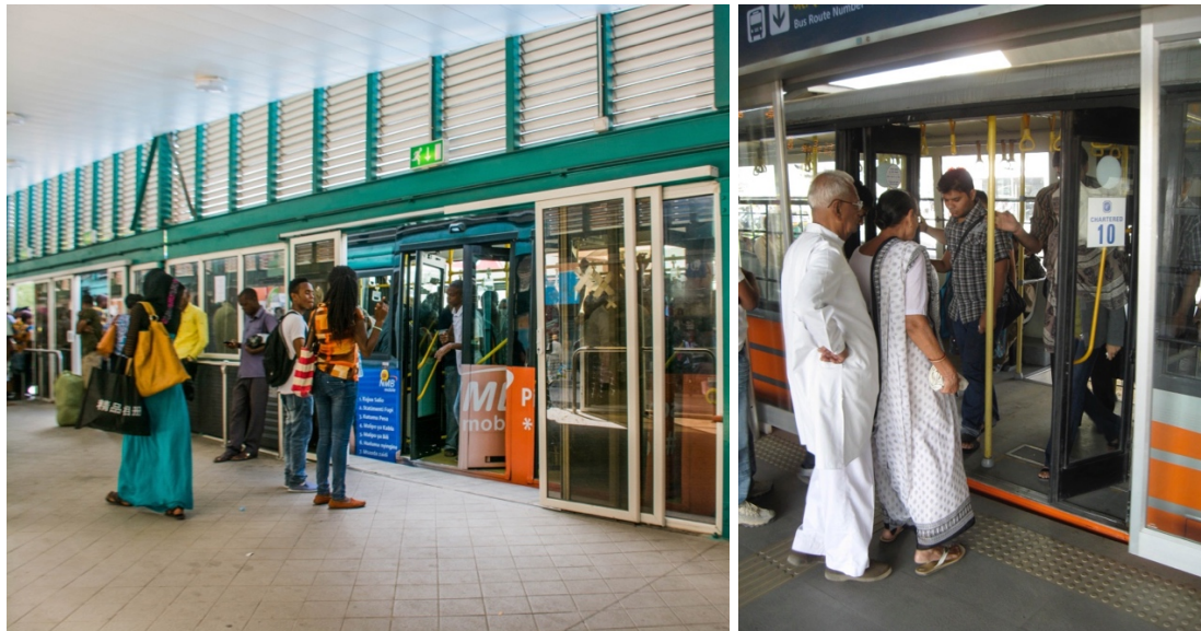
Figure 24: Level boarding has been applied in BRT systems in Dar es Salaam (left) and Ahmedabad (right) to facilitate faster boarding and alighting and universal accessibility.
