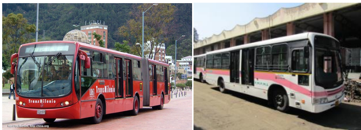
Figure 26: Wide doors on the station side of buses allow for fast boarding and alighting: 18 m articulated bus in TransMilenio, Bogotá (left) and a 12 m bus in Rainbow, Pune (right).
