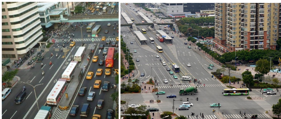
Figure 19: Station placement exactly at the intersection results in operational inefficiency in Taipei, Taiwan (left). A station shifted away from the intersection allows buses to queue at the intersection without blocking the docking bays in Guangzhou, China (right).
