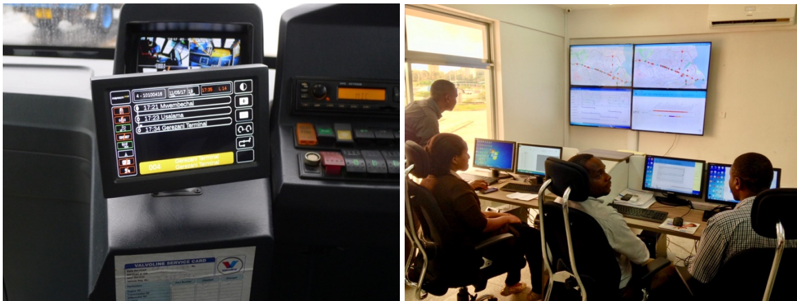
Figure 41: The Dar es Salaam BRT system employs an automatic vehicle location system to optimise bus headways.
