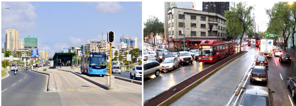
Figure 9: Median alignment secures BRT speed, capacity and service quality and is a defining feature of successful BRT systems across the world, including the DART BRT in Dar es Salaam (left) and the Metrobús BRT in Mexico City (right).
