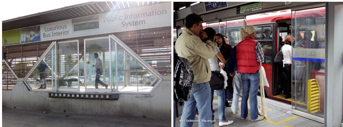
Figure 27: Platform screen doors improve safety and reduce fare leakage.
