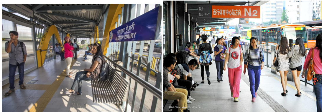
Figure 30: BRT stations should offer seating, leaning bars, and adequate circulation space to meet expected passenger demand: Rainbow, Pimpri-Chinchwad, India (left) and Guangzhou BRT (right).
