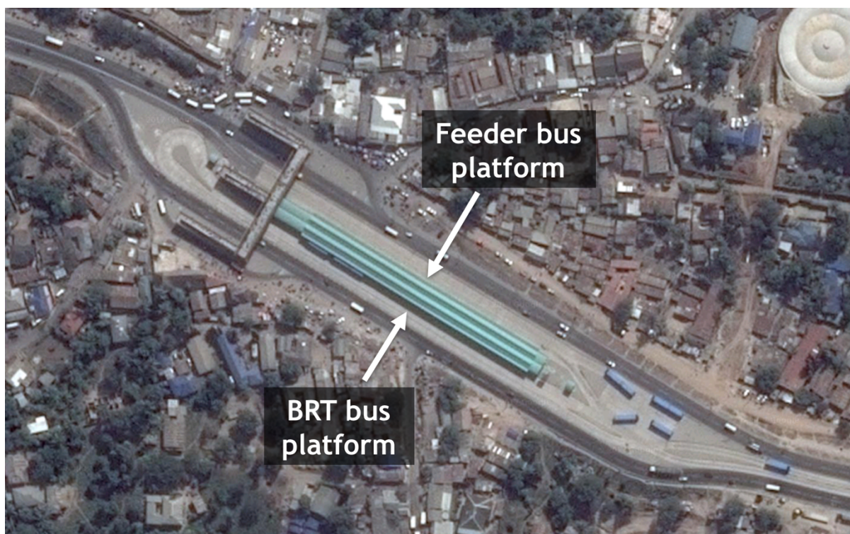
Figure 34: Dar es Salaam BRT system's Kimara terminal offers cross-platform transfers from BRT to feeder buses. The level of both platforms is the same to improve accessibility.
