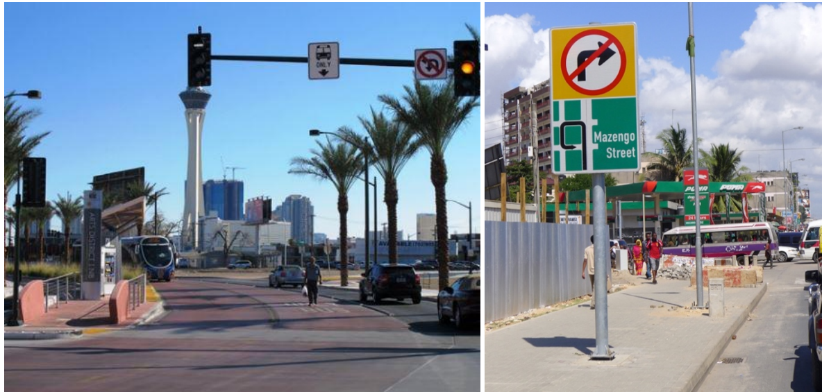
Figure 13: Forbidding turns across the bus lanes increases bus speeds at intersection: Las Vegas BRT (left) and DART BRT, Dar es Salaam (right).
